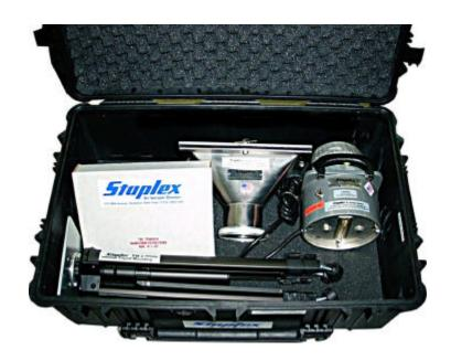
No. TF-CCK Carrying Case shown with accessories: Staplex Model TFIA Series High Volume Air Sampler, SH810 8"x10" Filter Holder Assembly, TR-1 Tripod Mounting, and Filters (accessories not included).
